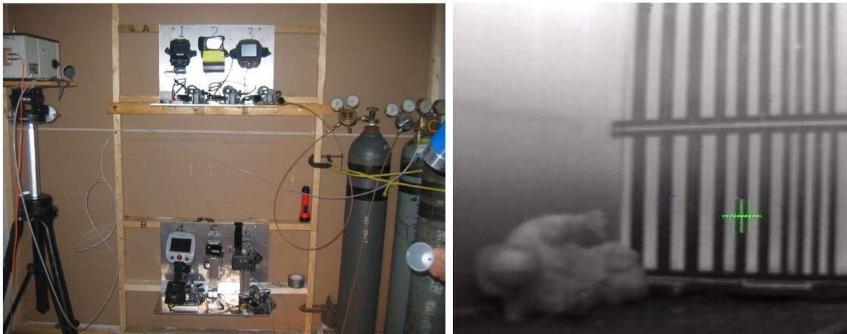
**Figure 5—4.** The TIC were mounted on shelves which were repositioned midway through the tests (left). Two bar targets were used, one in the upper layer and one in the lower layer, along with a heated mannequin in fire fighter turnout gear, shown in infrared (right).
