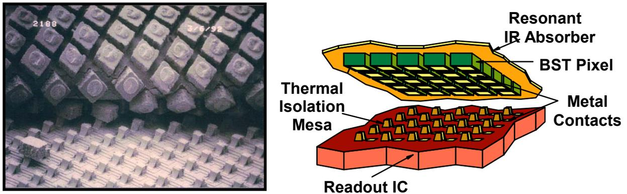
**Figure 2—5.** Hybrid Pyroelectric BST Detector. This is a solid-state ceramic detector that spontaneously polarizes when exposed to thermal energy [4].
