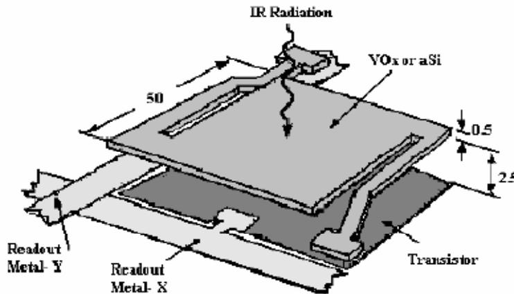
**Figure 2—6.** Microbolometer. This is an array of individual sensors, each of which generates a small portion of the overall thermal scene. The sensor material is either vanadium oxide or amorphous silicon [11].
