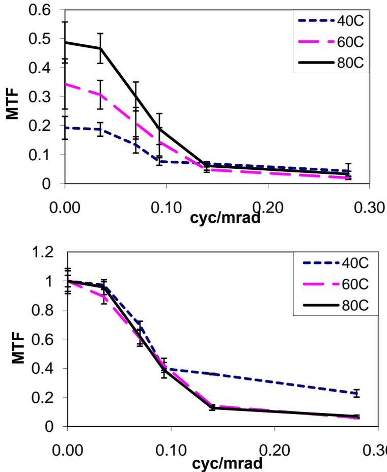
**Figure 7—8.** Illustration of the temperature independence of the spatial resolution measurement. The temperatures are indicated in Celsius. Once the original values (top) are normalized (bottom) the effect of image contrast (temperature difference) can be eliminated. The line for 40 °C on the right does not follow the other trends because there needs to be a minimum contrast in the knife edge image.
