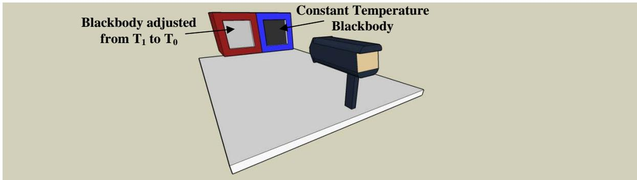
**Figure 6—11.** Experimental setup for thermal sensitivity test. The two blackbodies are adjusted until they both have the same luminance on the TIC display. Then one blackbody temperature is slowly decreased until a 2 % difference in luminance is observed between the two blackbodies.
