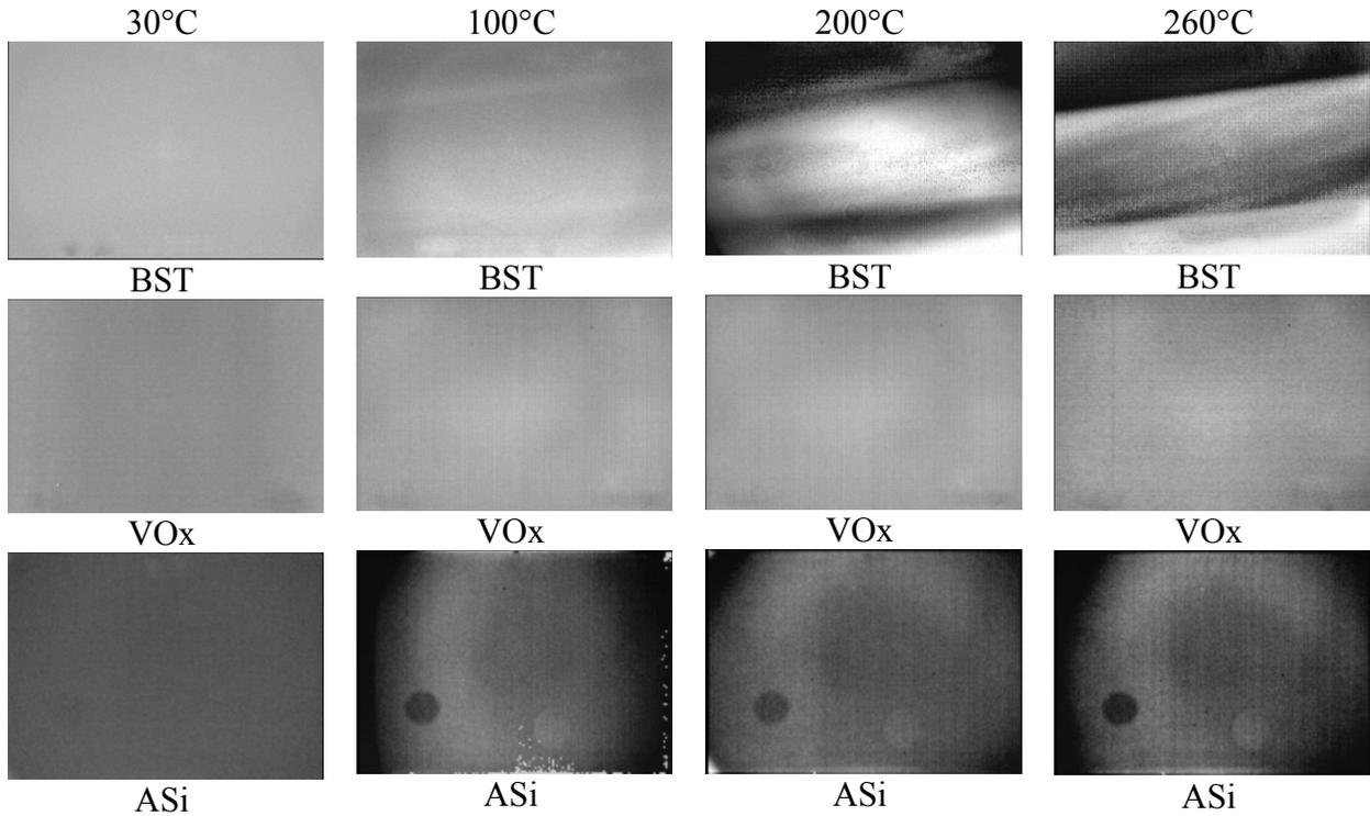
**Figure 7—4.** Actual nonuniformities observed from three different TIC at a variety of temperatures. BST, VO<sub>x</sub>, and ASi detector technologies are all represented along with a variety of different nonuniformities present in these cameras.
