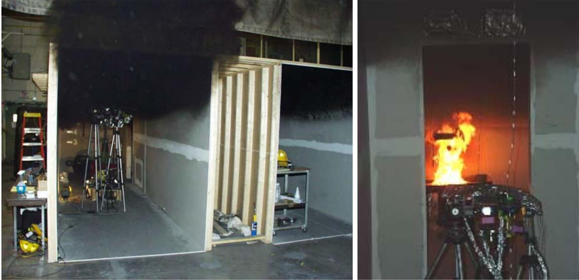
**Figure 5—2.** TIC are positioned in the hot upper layer viewing a target through heavy toluene smoke, test configuration D (left), and in the lower layer viewing flames and high heat conditions, test configuration A (right).
