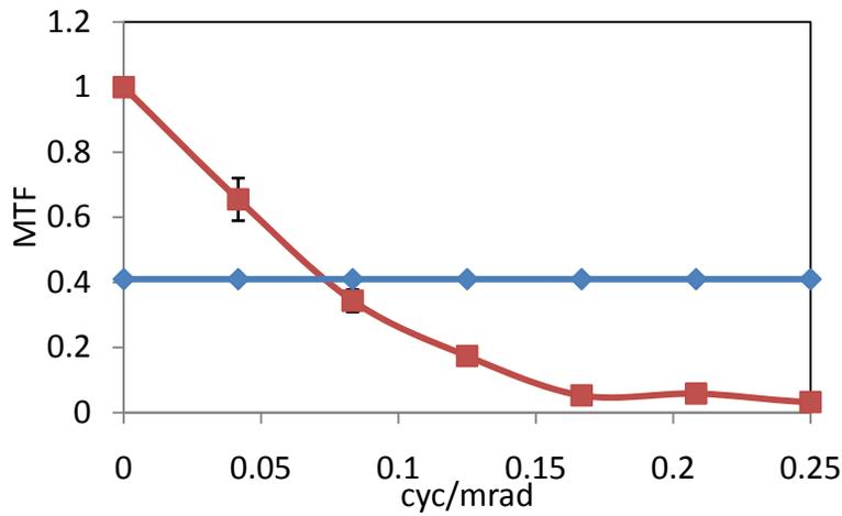
**Figure 7—7.** Comparison of the spatial resolution of the BST, VOx, and ASi TIC. The SFR value given for each camera technology represents the area between the MTF curve and Nonuniformity. The spatial resolution measurement for each camera is dependent upon the nonuniformity measurement as well.
