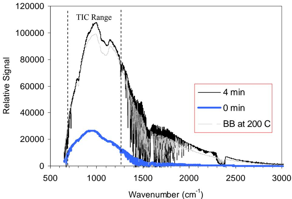
**Figure 5—12.** The relative FTIR signal measured at two times during an experiment burning carpet, padding, and wood. For comparison, measurement of the relative signal of a blackbody source at 200 °C ( $\pm 5$  °C, as per manufacturer’s documentation) is also shown.
