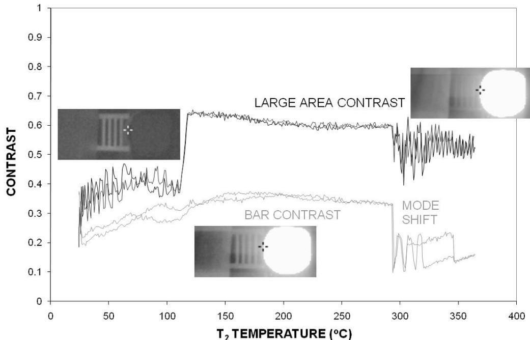
Figure 7—1 to Figure 7—3 as a function of  $T_2$  temperature; there are two tests shown in each graph.  $T_2$  is the temperature of a surface of area large enough to cause the TIC under test to shift
