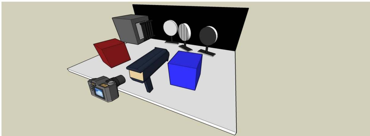
**Figure 6—5.** Alternative test setup for contrast and effective temperature range. When space is an issue mirrors may be used to redirect the thermal radiation to the TIC. The results presented in this paper were obtained in this configuration.
