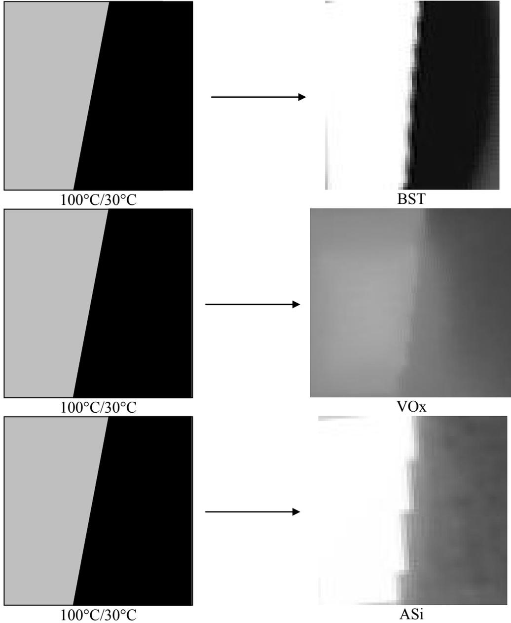
**Figure 7—6.** Illustration of how of how three different cameras interpret the same ‘knife edge’ thermal target. The three different cameras have different sensor technology, but also have different pixel resolutions (320x240, 160x120, and 160x120 respectively), optics, and internal image processing that affects the spatial resolution of the image on the display. The analysis of these images is presented in Figure 7-6.
