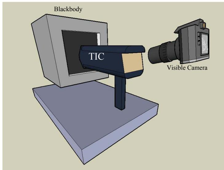
**Figure 6—7.** Test setup for measuring the nonuniformity of a TIC. The TIC is placed close to the surface (~5cm) of a uniform large area blackbody surface. The temperature is increased and the images are taken by the visible camera to determine image nonuniformity.
