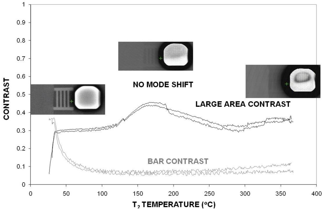
**Figure 7—2.** Plots of large area contrast and bar contrast data used to determine image contrast and effective temperature range of a TIC using an BST, 240 x 320 detector array. Test results for two tests are shown.
