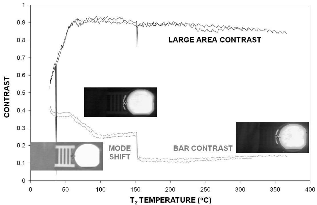
**Figure 7—3.** Plots of large area contrast and bar contrast data used to determine image contrast and effective temperature range of a TIC using an VOx, 120 x 160 detector array. Test results for two tests are shown.
