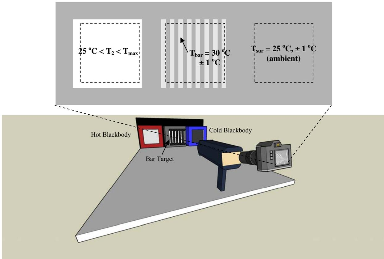
**Figure 6—4.** Test target setup used for the contrast and effective temperature range tests. For large area contrast, the bars in the middle of the test target are ignored. The standard deviation of the combined pixel intensities within the dashed areas on the left and right side of the test target are calculated, then divided by the *Bitdepth* to determine the contrast as a function of  $T_2$ , which changes from  $25\text{ °C}$  to  $T_{\max}$ .
