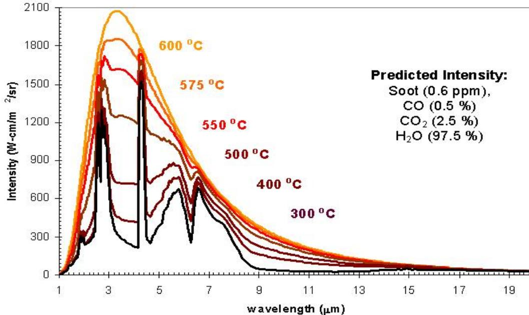
**Figure 2—2.** Predicted radiation intensity through a 12.7 cm (5 in) path length for a simulated combustion atmosphere consisting of 0.6 ppm soot, 0.5 % CO, 2.5 % CO<sub>2</sub>, and 97.0 % H<sub>2</sub>O [9]. The media temperature is held at 600 °C and the wall temperature varies from 0 °C to 600 °C.
