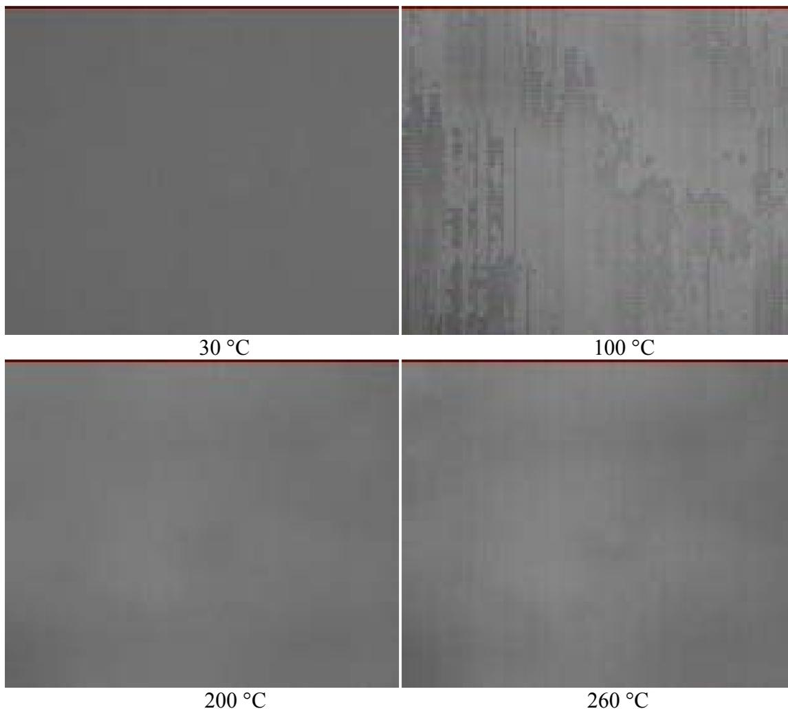
**Figure 6—8.** Variation in nonuniformity of a TIC with increasing temperature. As the test target temperature increased, nonuniformities became more apparent. The TIC shifted to a less thermally sensitive mode between the 100 °C and 200 °C images.
