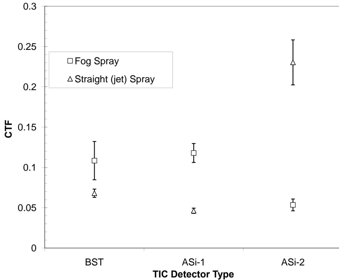
**Figure 5—14.** *CTF* of a thermal target viewed by three TIC through fog and straight (jet) sprays with a 2.2 MW fire in the field of view. The error bars represent the standard deviation of the *CTF* with a coverage factor of 2 (95 % confidence).
