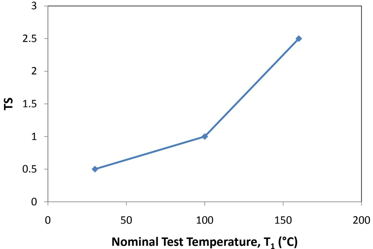
**Figure 7—9.** Example thermal sensitivity response for a characteristic TIC. A smaller value for thermal sensitivity indicates that the camera is more sensitive to small differences in temperature. The thermal sensitivity increases with increasing nominal temperature due to a larger contrast necessary for the user to perceive a temperature difference.
