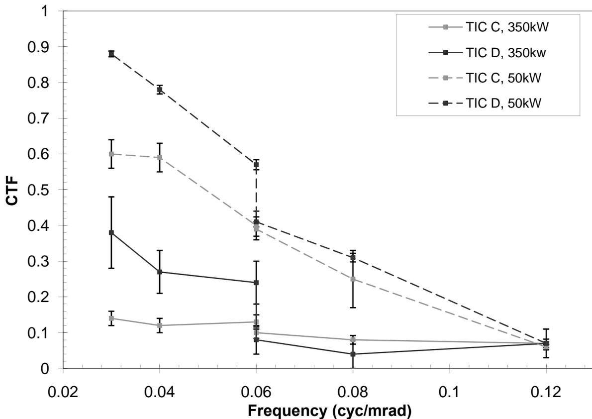
**Figure 5—7.** Comparison of heat effects, VOx detector technology.
