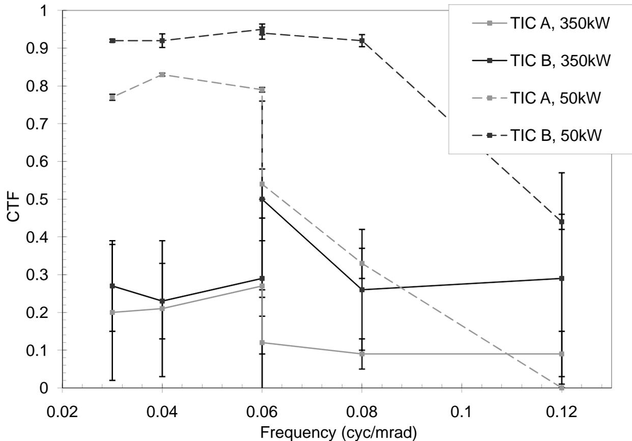
**Figure 5—6.** Comparison of heat effects, BST detector technology. These two TIC differ only in age, both having a 320 x 240 detector array. (where applicable uncertainties are determined statistically as stated in section 7.5 and reported with a coverage factor of k=2)
