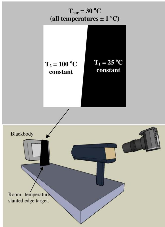
**Figure 6—9** Slanted edge spatial resolution test target. The slant is  $5^{\circ}$  from vertical, the hot and surrounding temperatures are held constant throughout the test. The target dimensions are at least 15 cm in each direction. All surfaces in the field of view have  $\epsilon \geq 0.94 \pm 0.002$ .
