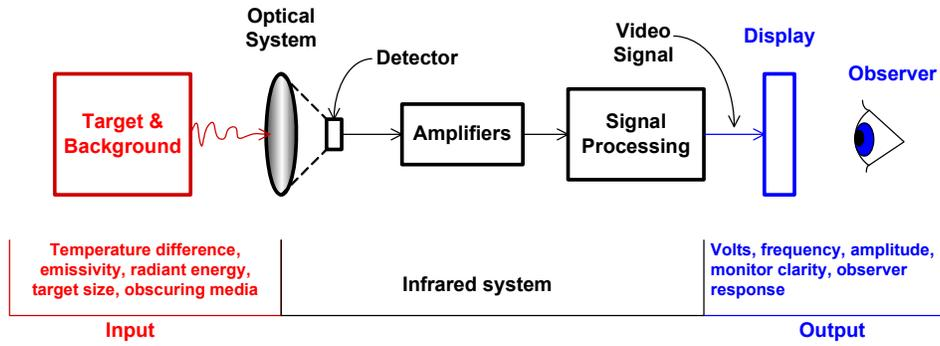
**Figure 2—4..** Generic schematic of major TIC design components.
