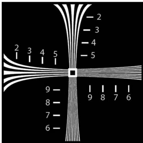
**Figure 6—1.** Reflective test target used for image recognition tests. The test target dimensions are 61 cm (24 in.) in each direction. The white markings shown here are highly reflective foil with an  $\epsilon \leq 0.1$  and the background is foam core with a black matte finish having an  $\epsilon \geq 0.9$ .
