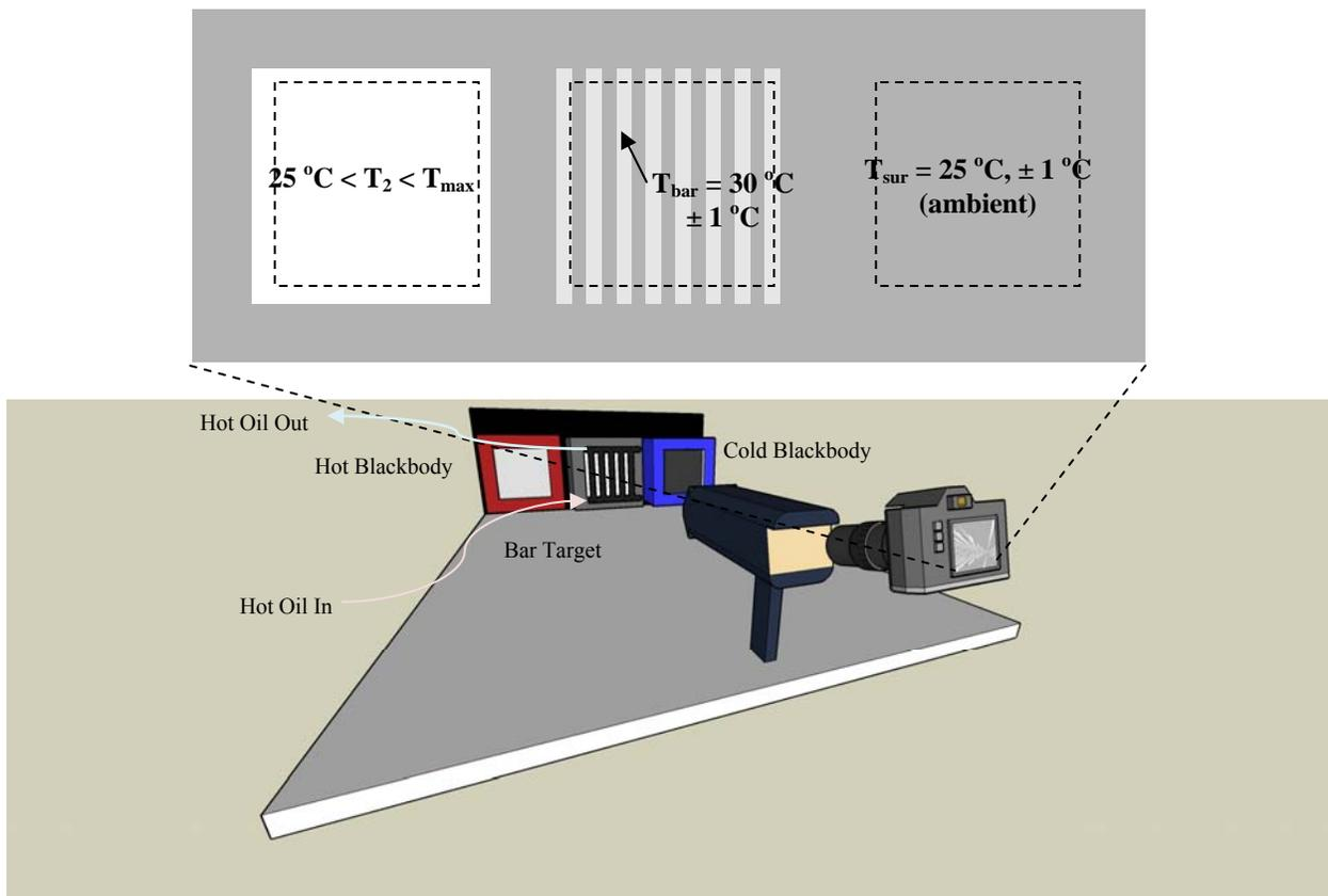
**Figure 6—6.** This test target is used for the contrast and effective temperature range tests. For the effective temperature range, the contrast of the central area, which incorporates bars having a constant temperature difference, is measured while the hot blackbody surface temperature ( $T_2$ ) increases.
