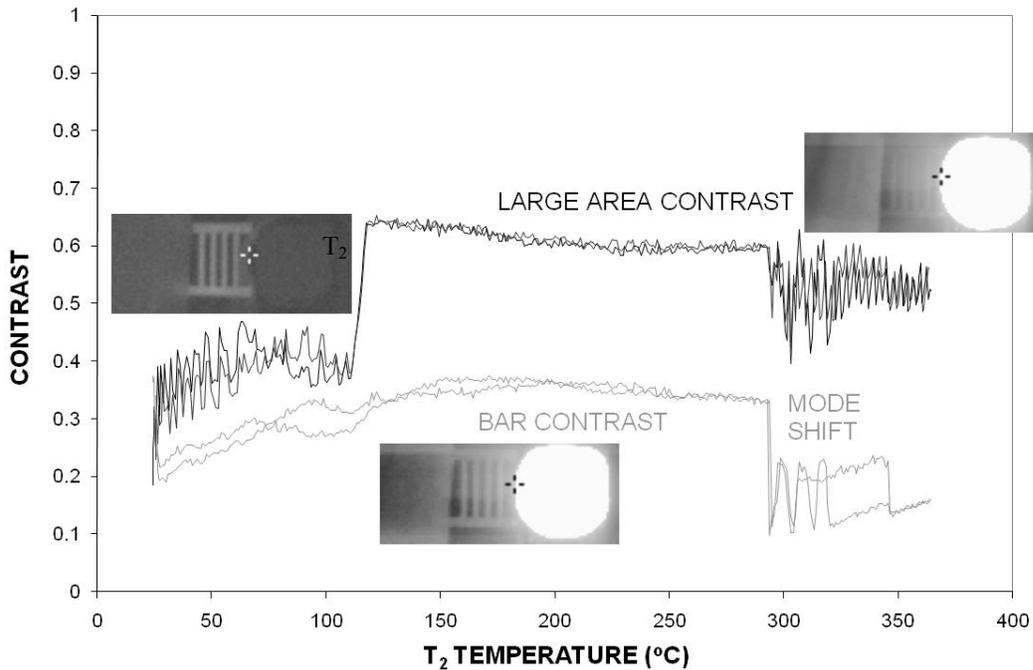
**Figure 7—1.** Plots of large area contrast and bar contrast data used to determine image contrast and effective temperature range of a TIC using an ASi, 120 x 160 detector array. Test results for two tests are shown.
