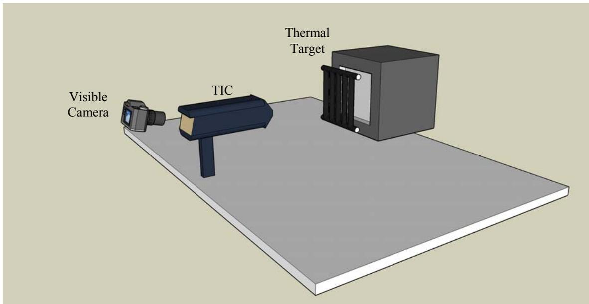
**Figure 6—3.** Schematic diagram of image capturing setup. As the TIC views a thermal target, a high resolution visible camera is focused on the TIC display. A mounting bracket (not shown) is to be provided by the TIC manufacturer to optimally position the visible camera.
