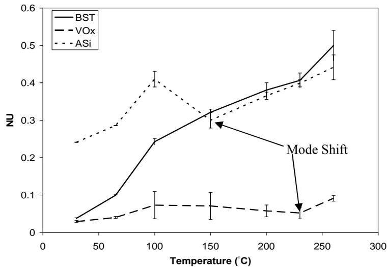
**Figure 7—5.** Image nonuniformity as a function of target temperature while looking at a uniform temperature surface. For the three specific TIC tested, the VO<sub>x</sub> TIC produced the least nonuniformity while the ASi and BST cameras had higher nonuniformities at different temperatures.
