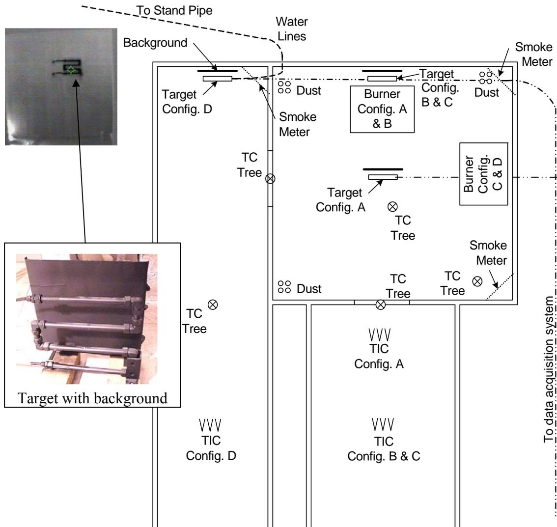
**Figure 5—1.** Plan view of Series 1 full-scale testing structure with inset showing the target and background. The target was placed on the floor in test configuration A and mounted on the wall 1.5 m from the floor in test configurations B, C, and D.
