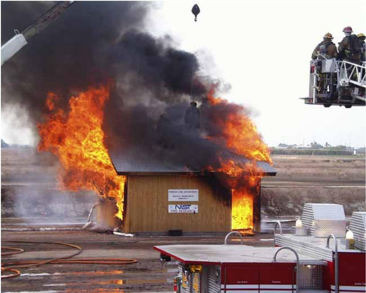
Figure 21. Photograph of test structure at 900 s after ignition when front door has burned away.
