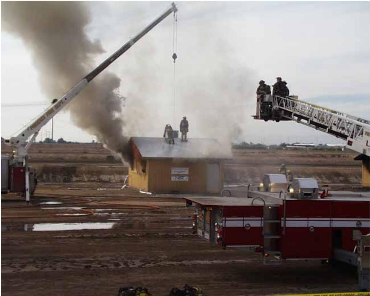
Figure 18. Photograph of test structure at 210 s after ignition.
