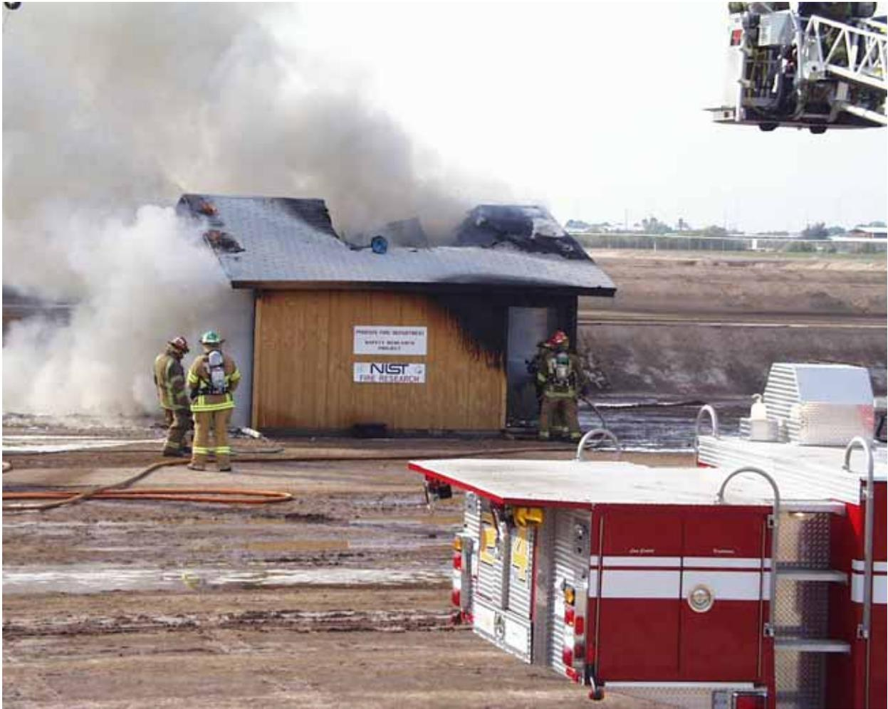
Figure 24. Photograph of test structure at 1140 s after ignition when suppression has been completed.
