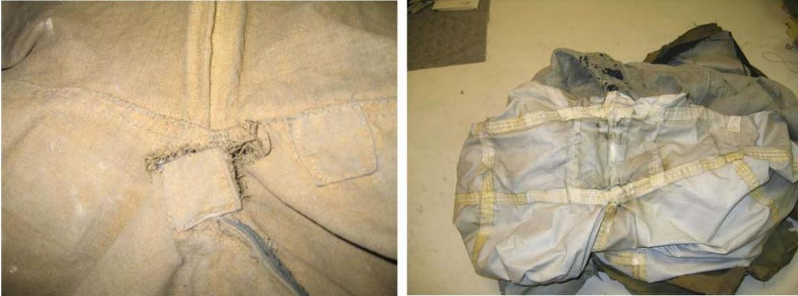
*Photo 3. The repaired crotch area of the turnout pants shell, and inverted liner with diminished thermal integrity due to age and use.*
