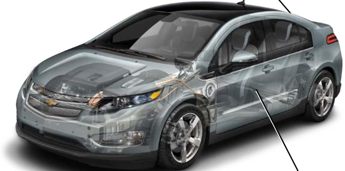
DO NOT CUT HERE. The Volt battery has 360 volt electrical potential at all times. It is inside the center tunnel and under the rear seat area.
