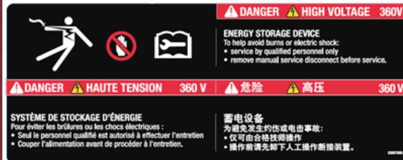
The high voltage warning labels are orange and indicate a potential shock hazard if high voltage is not properly disabled. The labels are located on all high voltage components with the exception of the high voltage battery which utilizes the danger label.
