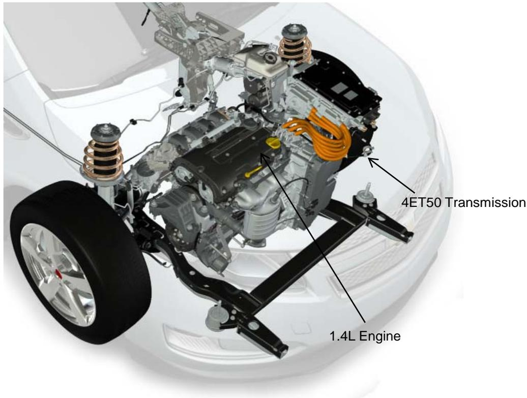
The 4ET50 transmission is a fully automatic, front-wheel drive transaxle, variable-speed, electronic controlled transmission. The transmission contains two electric motor / generators that are utilized to:
