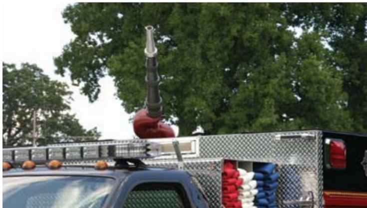
Above: The vehicle features a 2,000-gpm deck gun on top, as well as crosslays over the pump panel.
