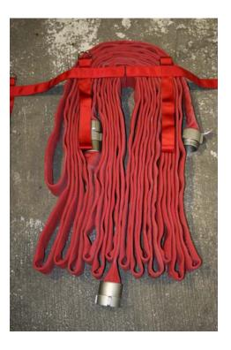
Tighten all the straps and make sure that the nozzle or the end of the male coupling is protected and secured to the carriers liking.
