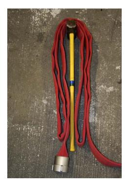
Continue packing the hose in this manner alternating the folds at the ends of the horseshoe 1-2 inches to enhance the lay of the hose. Connect the second section of hose and continue packing the hose. Care should be taken not to have the coupling on or near the top of the horseshoe as this will make carrying the pack difficult.
