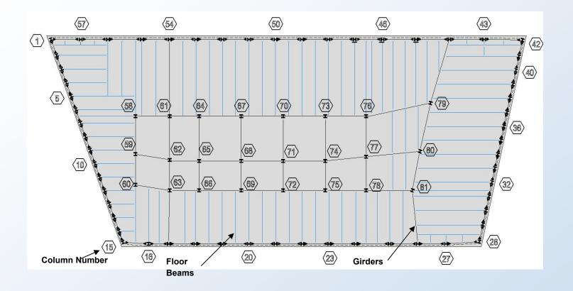
From the 7th floor to the 47th floor, WTC 7 was supported by 24 *interior columns* and 58 *exterior columns*. Columns 58 through 78 formed the building core. Columns 79, 80, and 81 were particularly large and supported long floor spans on the east side of the building.
