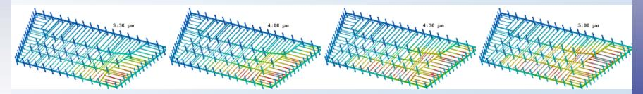
Temperature distribution (°C) on the floor beams of Floor 13.
