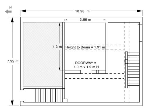
Figure 8. Plan view schematic of full-scale experimental arrangement
