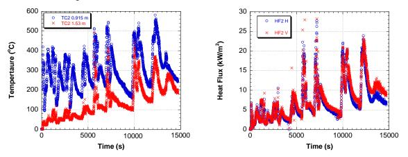
In the NIST Large Fire Facility, heat release rate (HRR) experiments, with the pallets set-up to represent fuel packages similar to those used in the last four evolutions, were conducted. The pallets were piled on edge into a corner composed of 2.44 m by 2.44 m walls covered with two layers of 13
